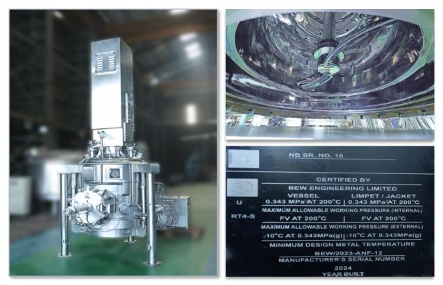
Pressure vessels that operate at pressures over 15 PSI are required to meet stringent ASME guidelines for safety and quality. The ASME "U" Stamp certifies that BEW's products adhere to these standards, ensuring that they are designed, manufactured, and tested to meet the highest levels of reliability and safety. The "U" Mark on BEW's equipment signifies compliance with ASME Section VIII Division 1, which sets the industry standard for pressure vessel design and construction.
