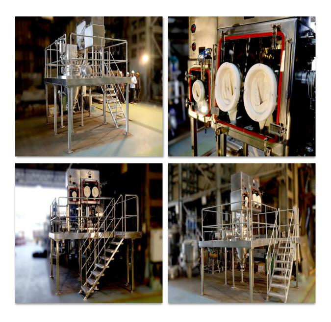
To meet the stringent requirements of handling potent materials, the mixer dryer is equipped with a Glove Box at its inlet. This setup provides a controlled environment, ensuring operator safety and product integrity. Key features of the Glove Box include:
