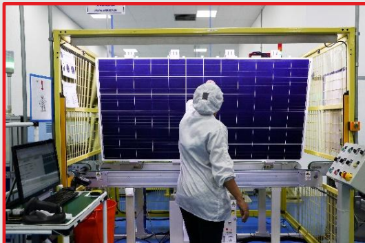
Final Visual Inspection
