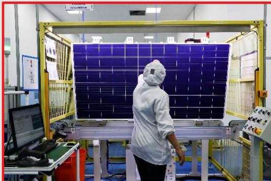
Final Visual Inspection
