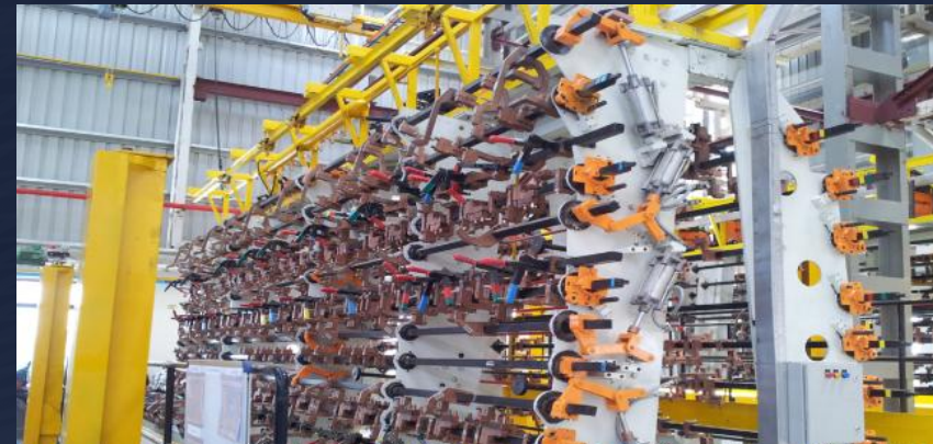
Bus Assembly Welding Fixture of size 12M
