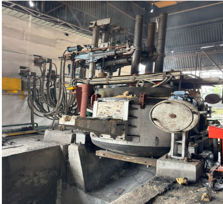
Newly installed PLC-based Electric ARC Furnace at Abha Power and Steel Limited's Bilaspur facility.
