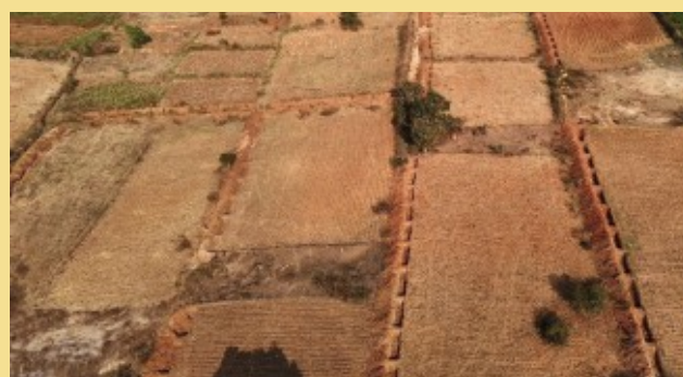
Trench Cum Bund at Chitikayathanhalli Village
