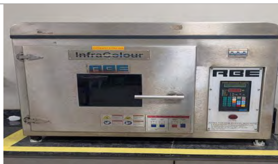
IR Dyeing Machine for Lab batch dyeing in Application Lab
