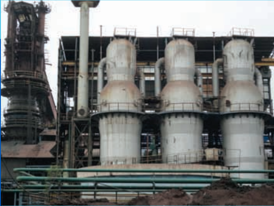
Hot Blast Stoves of Russain Technology installed at the MBF Plant
