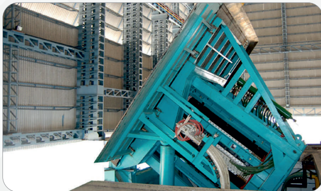
Induction Melting Furnace
