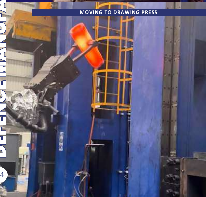
HOT PIECE AFTER DESCALING
