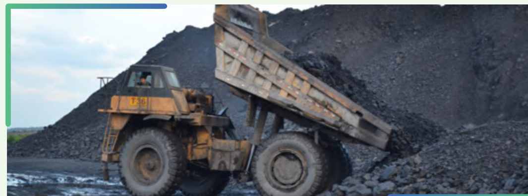
● Dumper unloading coal in the stock yard
