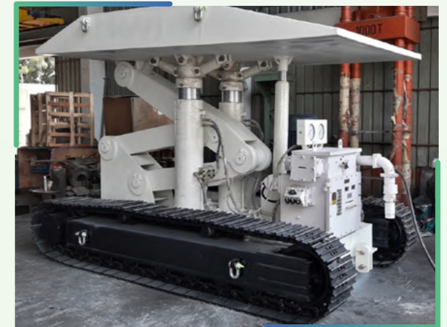
● Self-Advancing Goaf Edge Support (SAGES) currently under trial at Churcha Underground Mine, SECL
