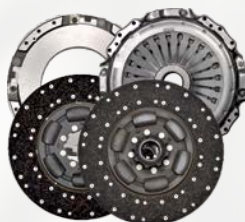
400mm Twin Diaphragm Spring
