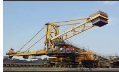
Stacker Reclaimer. Satpura TPP
