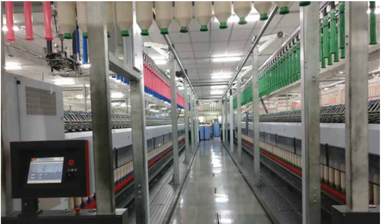
Zinser - 5 A Speed Frames with Auto doffing
