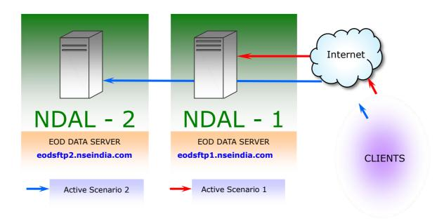
In NDAL premises, these two servers are available in active-active configuration. If one server stops responding, the clients are expected to switch over to the other server and vice-versa
